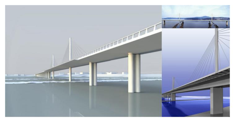
The total length of the Noia viaduct is 1,470m. It is divided into 46 spans of  $21.0m + 27 \times 30.0m + 48.0m + 102.0m + 48.0m + 14 \times 30.0m + 21.0m$ .
